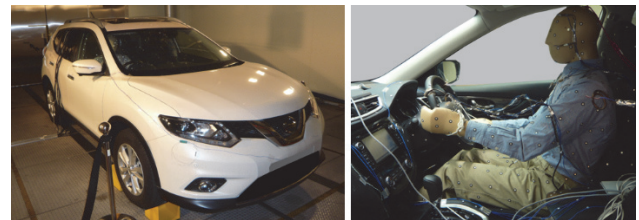
Fig.1 Vehicle (left) and thermal manikin (right) used for the experiment.
