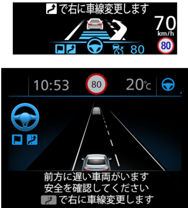
Fig.6 System's proposal for lane-change assistance
