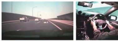
Fig.16 Driving simulator evaluation example: approval task for lane-change assistance to exit
