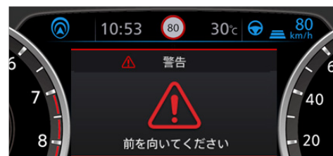
Fig.5 Driver-monitoring system and its warning for the driver to attend to the road ahead
