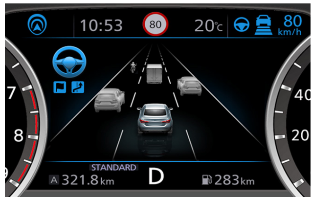
Fig.4 360° real-time surrounding display
