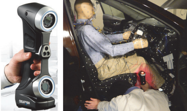
Fig.8 Measurements using 3D Handy laser scanner
