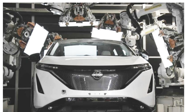
Fig. 7 Integrated automatic inspection of specifications and scratches
