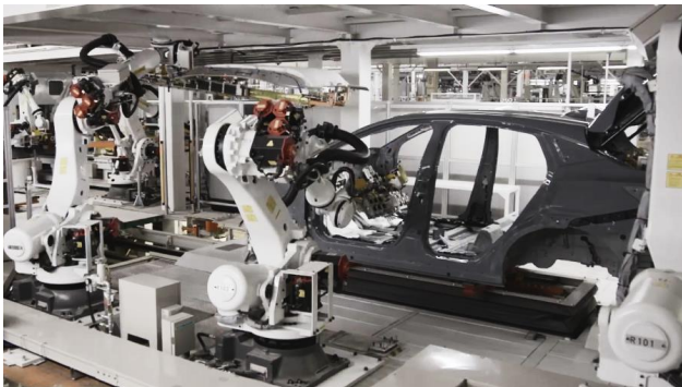
Fig. 8 Automatic headlining assembly
