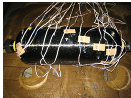
Fig. 5 Strain gages on tank No. 4 set up.
