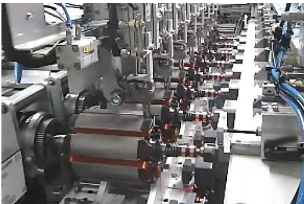
Fig. 5 Automation of magnet-free field motor winding
