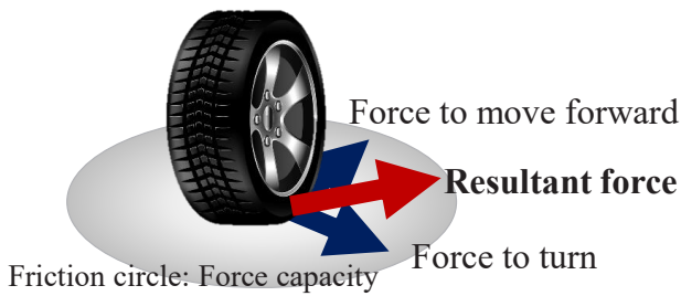
Fig.3 Tire friction circle and resultant force
