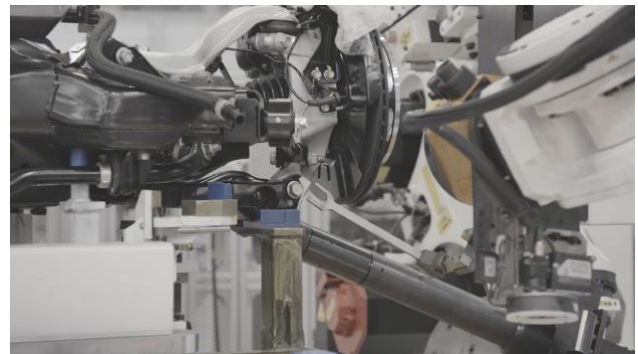
Fig. 6 Automatic tightening and alignment of suspension links
