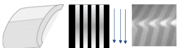
Fig.7 Fringe image differences due to combinations of character line and fringe pattern
