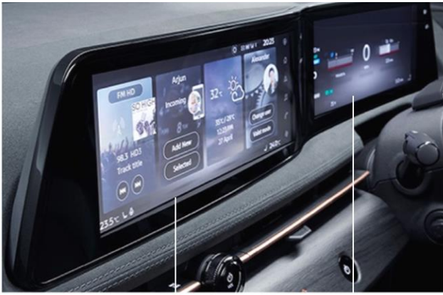
Infotainment display Meter display Fig.4 S-shaped display harmonized with the interior
