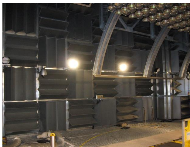
Fig. 8 Rainfall and snowfall test room with all-weather environmental chassis dynamometer
