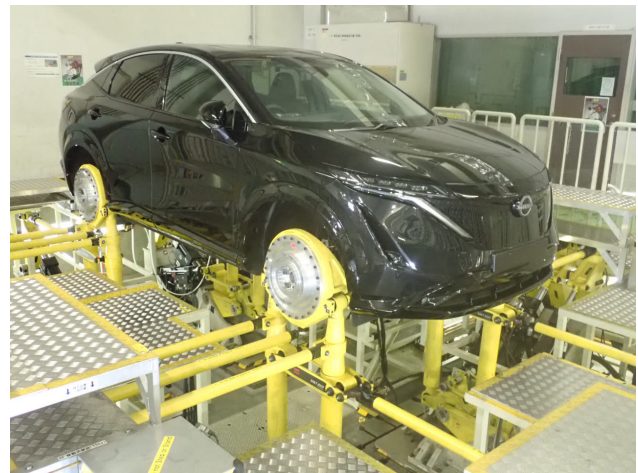
Fig. 3 Photograph of the road simulator (as an example of bench test equipment)
