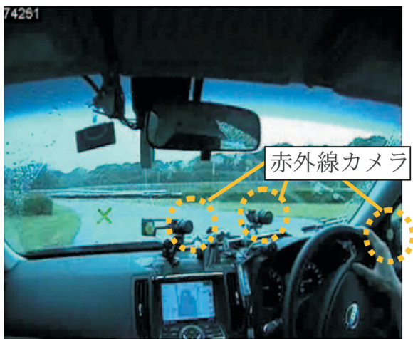
図-2 実験時車両装着状態 Fig. 2 Measuring equipments on board
