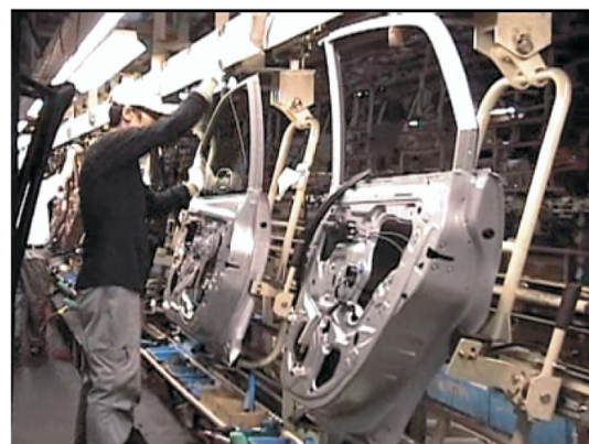
図-4 複雑な部品取付け軌跡を持つ組立作業例 (ドアガラス取付け) Fig. 4 Example of assembly work with complex parts set path (Door glass assembly)
