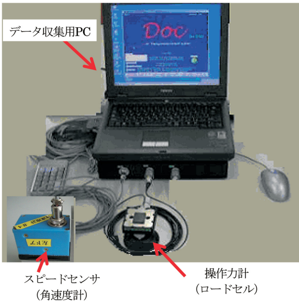
図-2 ドア閉じ計測装置 Fig. 2 Door closure measuring equipment
