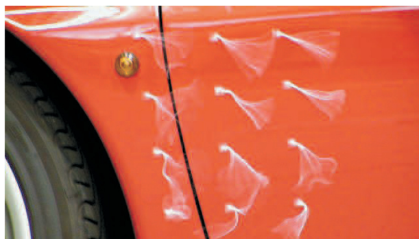
図-8 タフトを用いた流れの可視化 Fig. 8 Flow visualization with tufts on car-body
