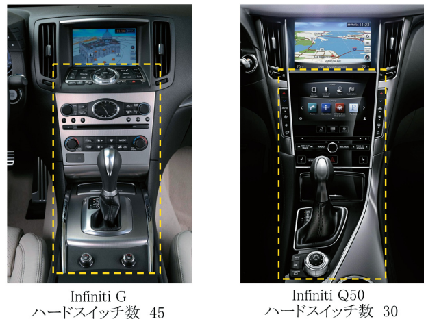
図-6 Infiniti GとInfiniti Q50のハードスイッチ数 Fig. 6 Number of switches of Infiniti G and Infiniti Q50
