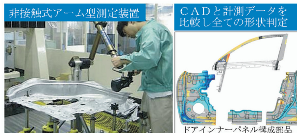
図-1 3次元形状計測装置と解析事例 Fig. 1 Examples of 3D measurement equipment
